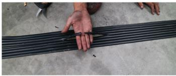
**STEP 6:** Push a joining barb onto one of the sides. Using a lubricant will make this easier.
