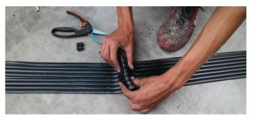
**STEP 1:** Squeeze the collector upward to expose the hole in the collector.
