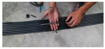
**STEP 4:** Cut the collector on either side of the hole to remove it.
