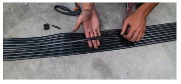
**STEP 3:** Expose approximately 5cm of collector around the hole.
